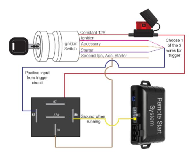
This will allow you to add a secondary Ignition, Accessory or Start wire to any of the CrimeStopper remote start and alarm.
